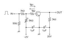
IC=10IB1=-10IB2=10mA For PNP, the polarity is reversed.
